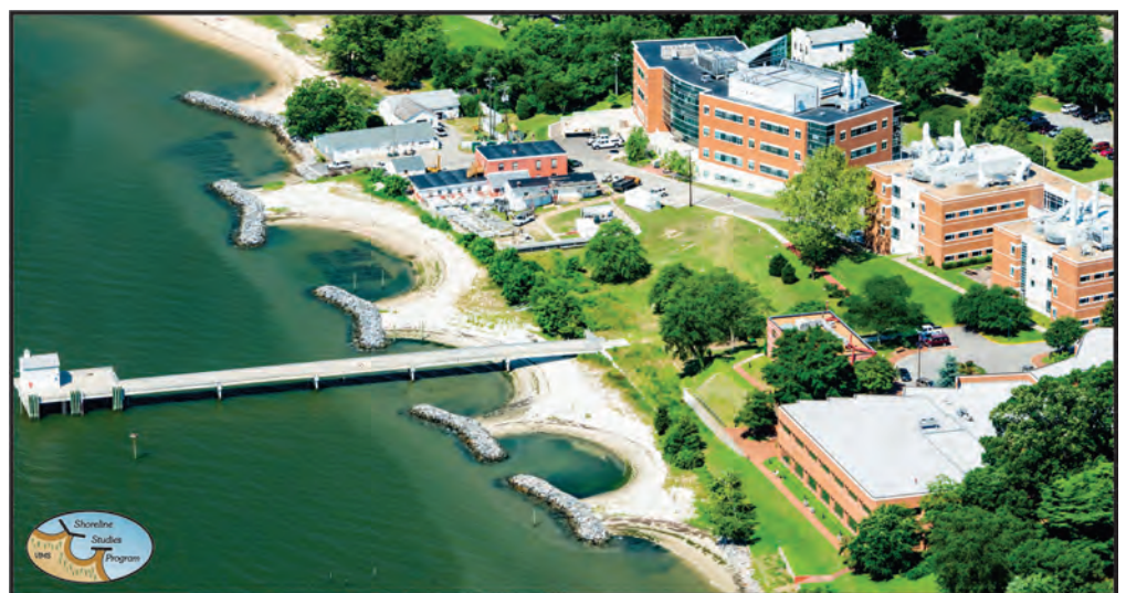
Figure 3-6. Aerial photo of breakwaters at the Virginia Institute of Marine Science campus on the York River. While the physical characteristics of breakwater sites differ, the goals are the same: protect the upland bank/marsh with a wide recreational/protective beach.
