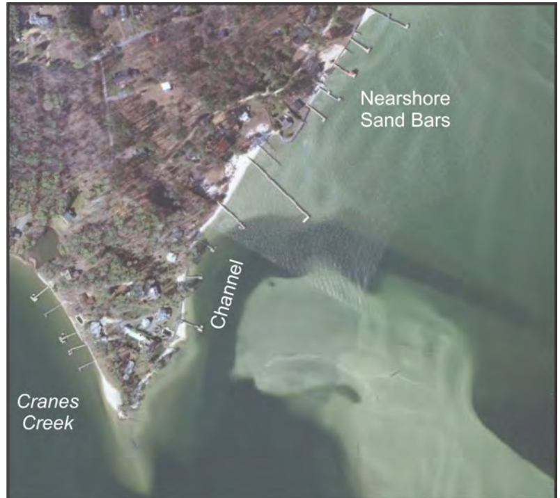
Figure 2-4. A VGIN 2009 photo shows the channel into Cranes Creek in Northumberland County, Virginia. Sand bars north of the channel will attenuate waves while the shoreline adjacent to the channel has no bars and will feel the full effect of the waves impacting the shoreline.
